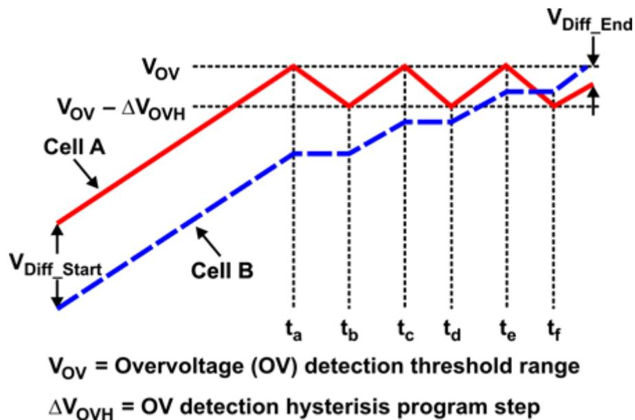
Figure 2 Example of automatic balancing algorithm
