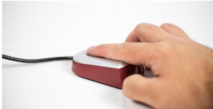
*Figure 5 Fingerprint login with the WF 2111 reader*
