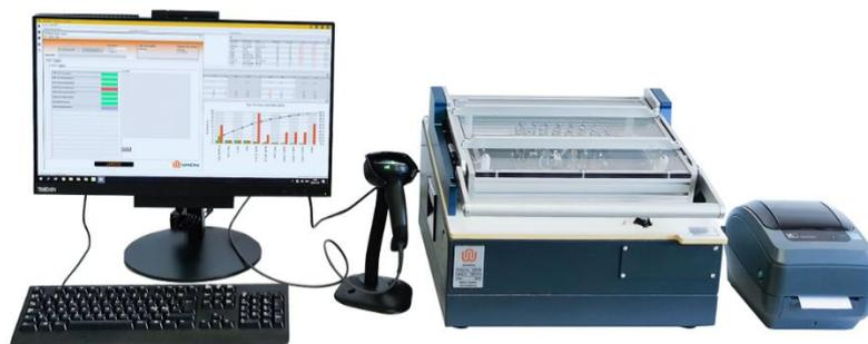
Figure 4 Test station with computer, barcode scanner, fixture and label printer
