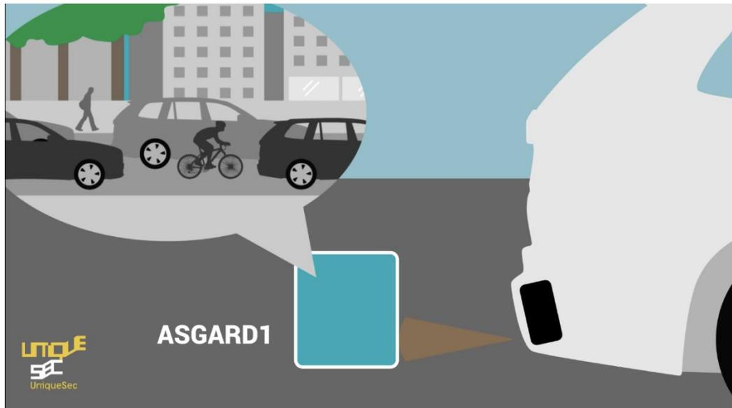
*Figure 1. Car radar detects objects simulated by the ASGARD1 system*
