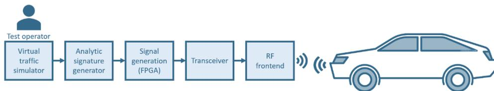
Figure 2. Block diagram of the radar test and verification solution
