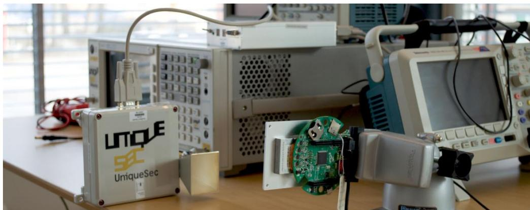
Figure 3. Lab setup of a radar and the ASGARD1 RF frontend
