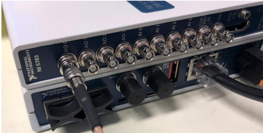
Figure 4. The FlexRIO FPGA and the Transceiver Adapter Module
