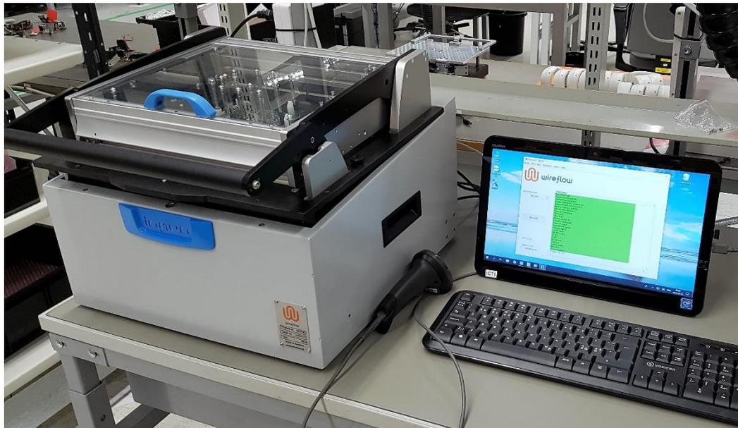
*Figure 4: Complete production tester setup with fixture to the left, hand scanner in the middle and the controller PC to the right.*
