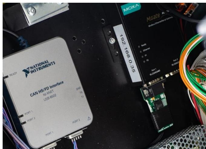
Figure 6 An I/O-box containing CAN and isolated RS232 interfaces
