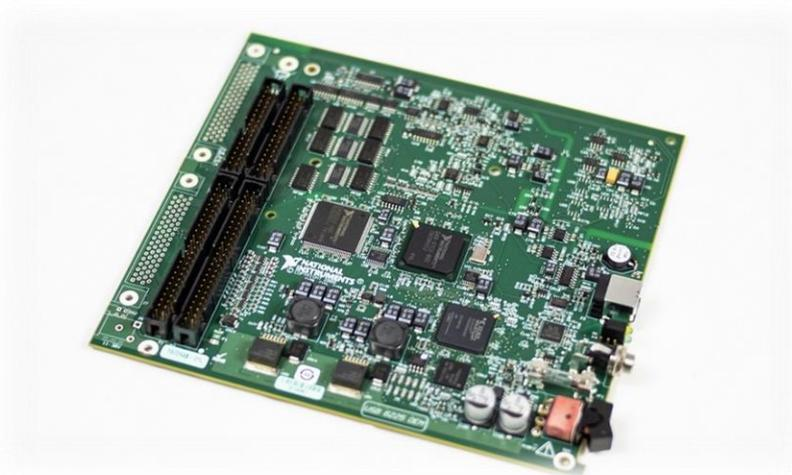
*Figure 1 The USB-6001 OEM Multifunction I/O Device from National Instruments*
