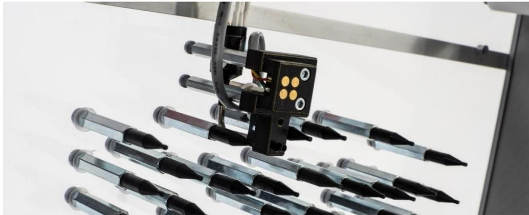
Figure 5 A light probe mounted on the pressure frame unit next to the pushrods
