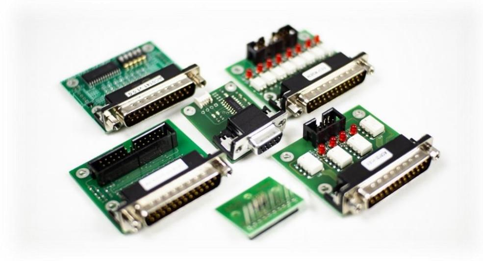
Figure 3 Signal conditioning boards, including three solid-state relay boards
